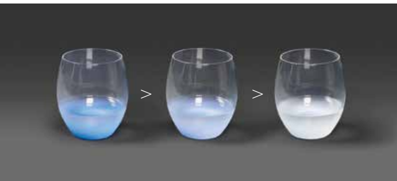
DEMONSTRATION OF THERMOCHROMIC WATER-BASED PAINT
