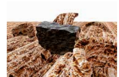
Silicon carbide grains cut through hard wood.
