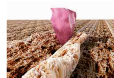
Aluminium oxide grains plough into soft wood types.
