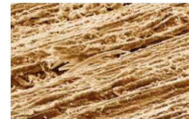
Wooden surface after sanding with aluminium oxide.
