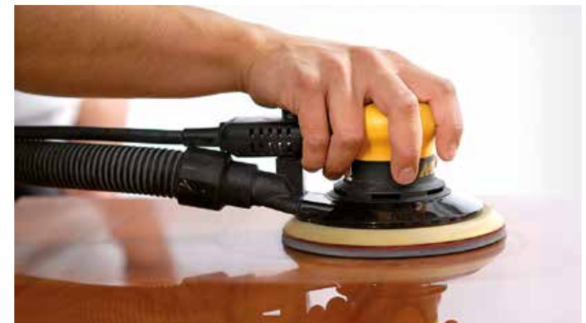
Sanding of top coat prior to polishing.
