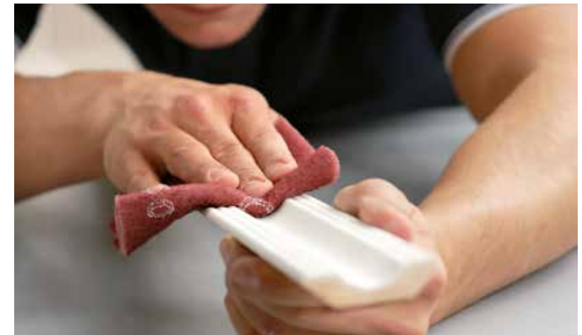
Intermediate sanding of paint or lacquer.
