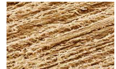
Wooden surface after sanding with silicon carbide.
